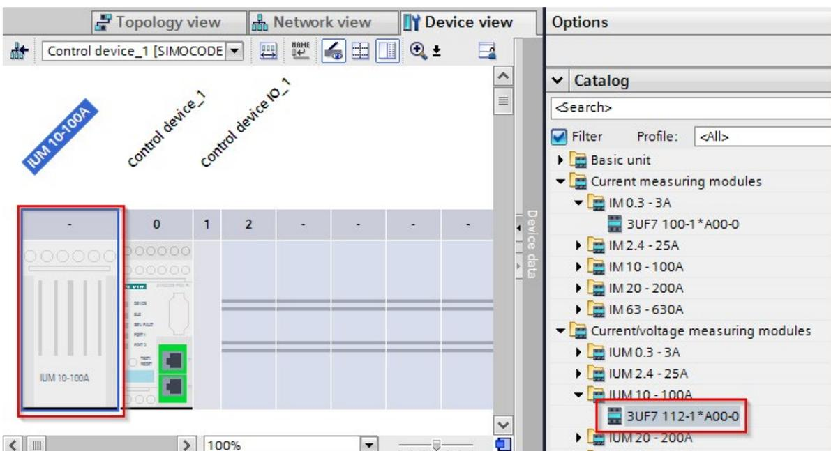
For communication via PROFINET IO, select basic type 3 at the SIMOCODE pro V in the inspector window "Properties" under "General > Module parameters > PROFINET parameters".
