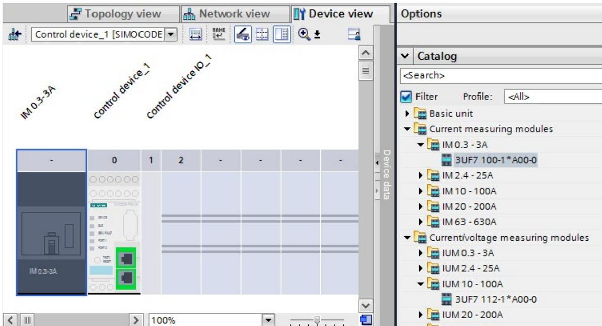
The figure below shows the corresponding IUM current/voltage detection module, e.g. "IUM 10 – 100A" in your application:
