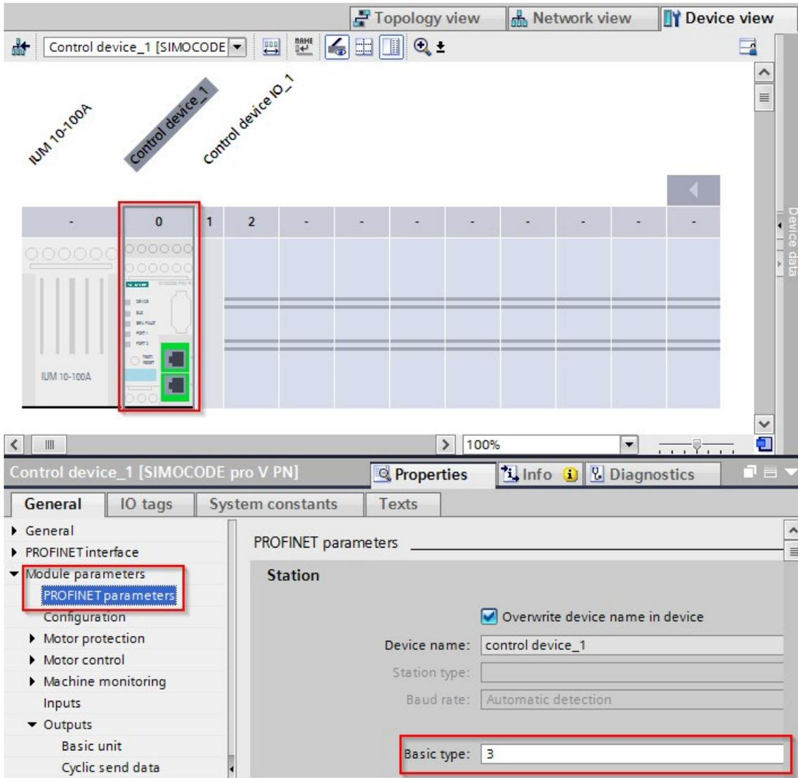
You can configure the selection of the cyclic energy data in the inspector window "Properties" under "General > Module parameters > Outputs > Cyclic send data". You configure the cyclic send data in the following sequence at the positions shown in the following figure:
