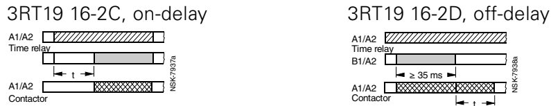
Fig. 3-45: Solid-state time relay block with semiconductor output, function diagrams (frame size S00)
