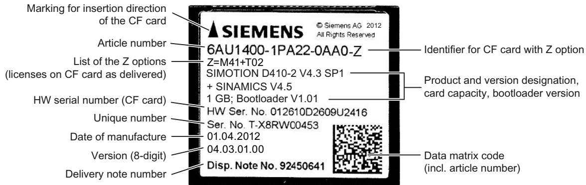
Figure 2-10 CF card (example of a 1 GB CF card)
