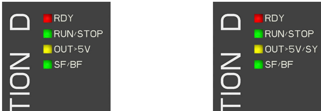
Figure 3-7 LED displays: D410-2 DP (on the left), D410-2 DP/PN (on the right)
