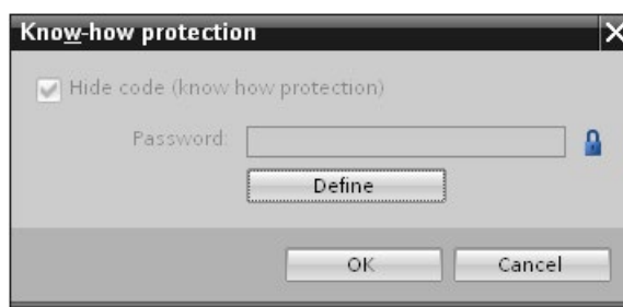
Figure 9-3 Setting up block know-how protection (2)
