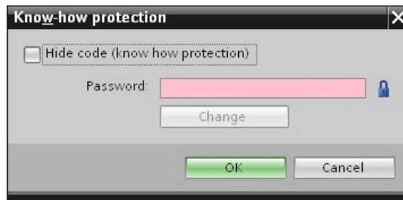
Figure 9-6 Removing block know-how protection (2)
