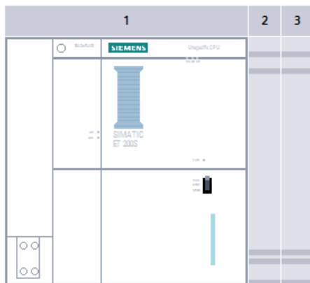
Figure 7-1 Unspecified CPU in the device view
